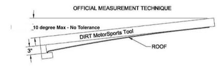
Do not take measurements at the top lid, as it will always be bigger to fit over the canister! The numbers will vary with different shape cells!
